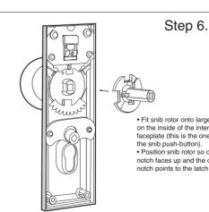
· Fit snib rotor onto large gear, on the inside of the internal faceplate (this is the one with the snib push-button). Position snib rotor so one notch faces up and the other notch points to the latch side.
